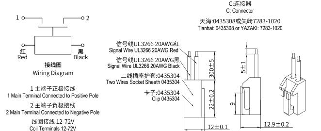
注:产品主触头按接线柱旁标示"1+"的连接负载"+"端,接线柱旁标示"2-"的连接负载"-"端 Note: The product main contact "1+" which is marked near the bolt is connected to the load "+" terminal, and "2-" is connected to the load "-" terminal.
