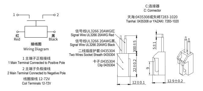
注: 产品主触头按接线柱旁标示 "1+" 的连接负载 "+" 端,接线柱旁标示 "2-" 的连接负载 "-"端 Note: The product main contact "1+" which is marked near the bolt is connected to the load "+" terminal, and "2-" is connected to the load "-" terminal.
